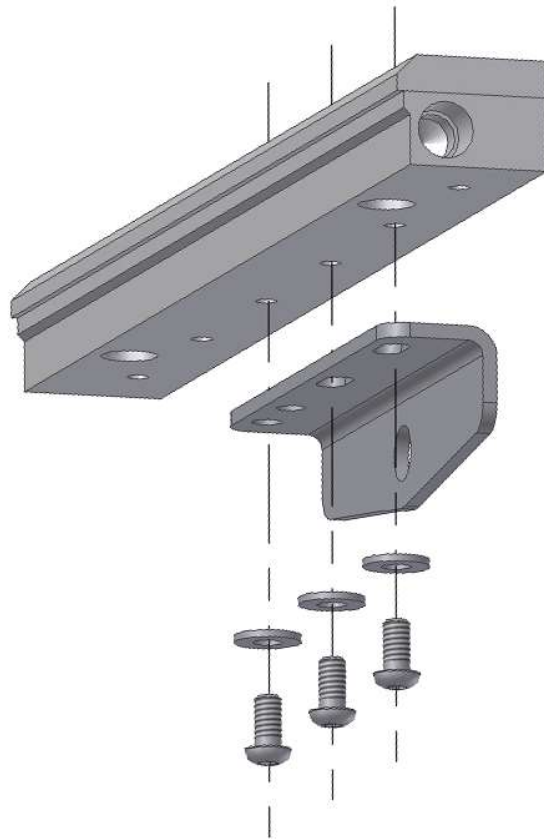
Figure 4 9" (229mm) St. St. Super Air Knife shown
